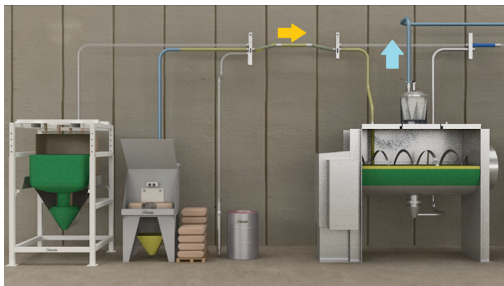
Fig. 9 – Mixer: a) introduction of the first product (above); b) introduction of the second product (below).
