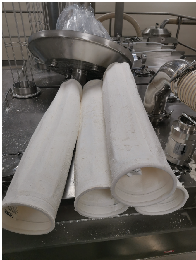
Fig. 10 - Disassembled bag / sleeve filter.
